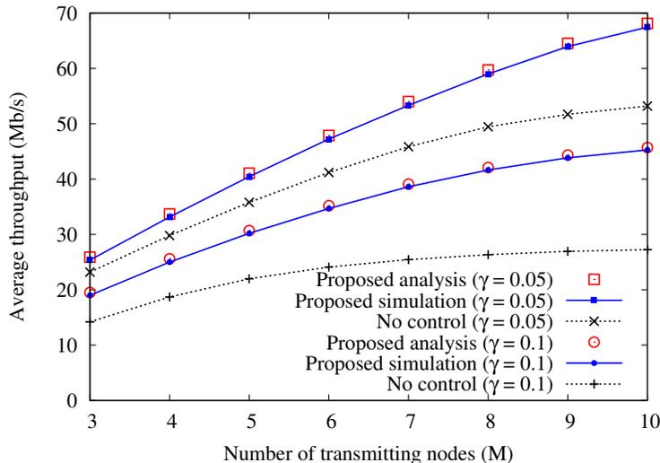
Fig. 2. Average throughput with respect to the number of transmitting nodes ( $\gamma = 0.05$  and  $0.1$ ).
