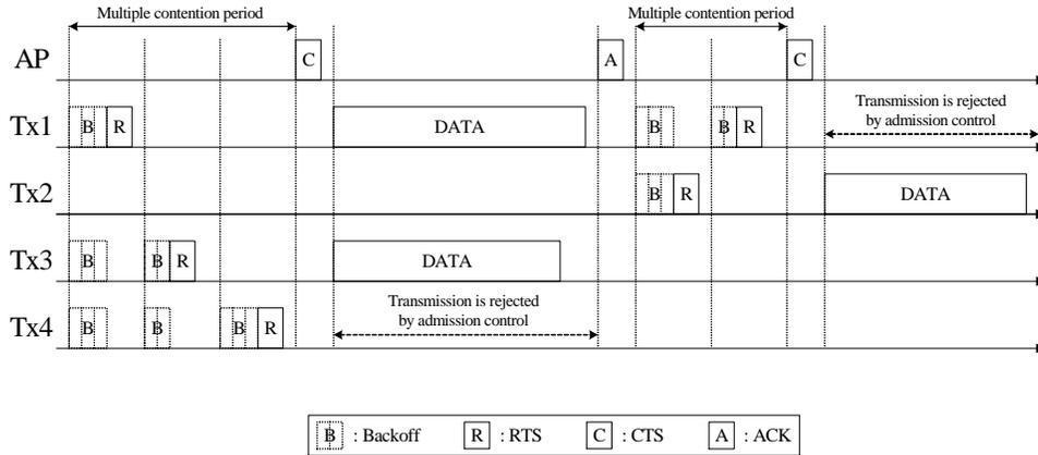
Fig. 1. Operation of a multiple-contention random-access scheme for an MPR system.
