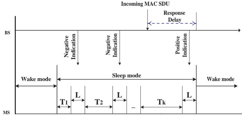
Fig. 1. Example of sleep mode operation in the IEEE 802.16e standard.
