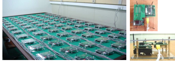
Fig. 2. IEEE 802.15.4 platform. Here, three components are combined using a 51 pin to 10 pin adapter. MIB600 is attached to MICAz and MTS300 to provide remote control functionality and auto-collection.
