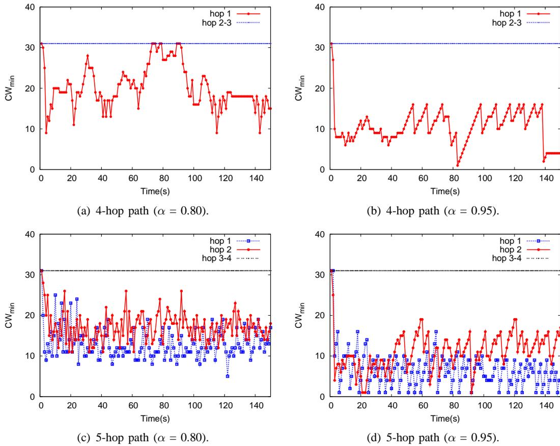
Fig. 5. Variation of  $CW_{min}$  with respect to time in the 4-hop and 5-hop wireless paths.
