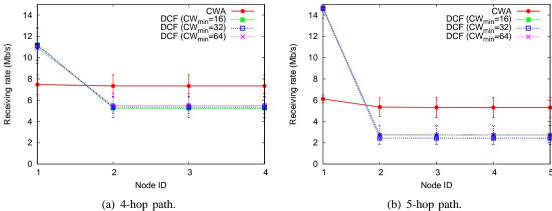
Fig. 3. Experimental throughput performance for IEEE 802.11 DCF and the proposed adaptive contention mechanism (CWA).
