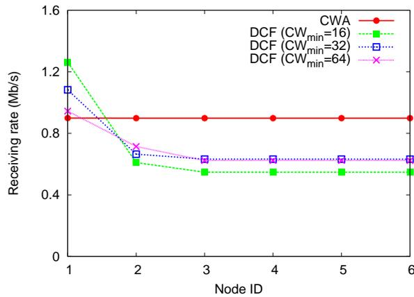
Fig. 2. Receiving traffic rate at each relay node on a 6-hop wireless path for a fixed, single  $CW_{\min}$  and an adaptively selected  $CW_{\min}$ . (The receiving rate at the last node is the end-to-end throughput of the multihop wireless path.)
