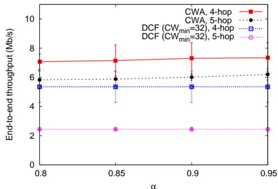
Fig. 4. Experimental throughput performance with respect to  $\alpha$  in the 4-hop and 5-hop wireless paths.
