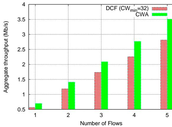
Fig. 6. Simulation result for the aggregate throughput performance with respect to the number of flows in a random topology.
